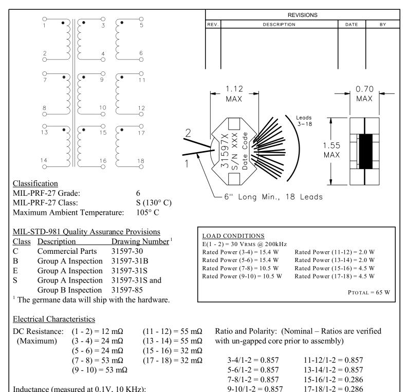
Inductance (measured at 0.1V, 10 KHz): (1 - 2) = 60  $\mu$ H ± 25% IDC = 3.9ADC
